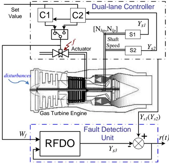
Fig. 1. Dual-lane control of gas turbine engines. Controller C1 and sensor S1 compose the primary lane. Controller C2 and sensor S2 compose a spare lane and is waiting in "hot back-up." When the primary lane fails, the spare lane comes online immediately. The model works as the third virtual lane.
