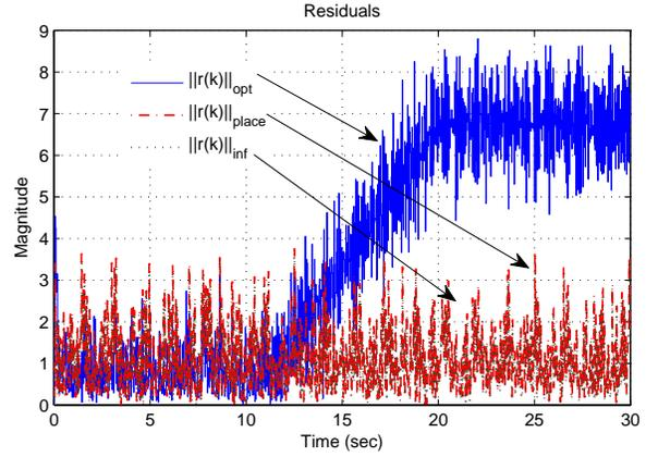
Fig. 6. Residuals of  $K_{opt}$ ,  $K_{place}$  and  $K_{inf}$  in the case of a saturated incipient actuator fault.
