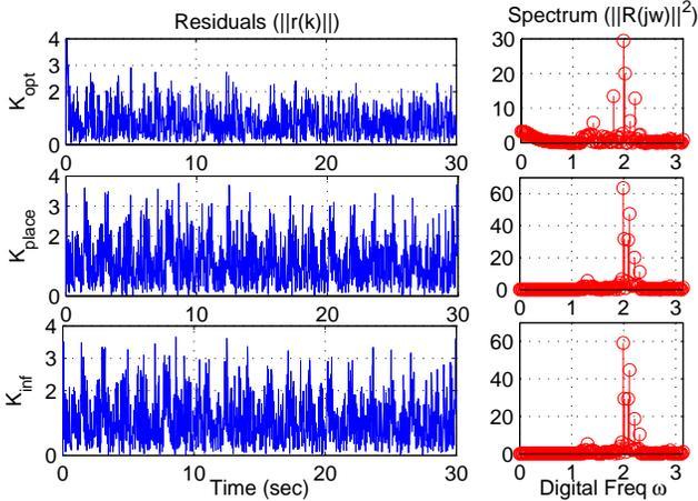
Fig. 5. Residuals  $\|r(k)\|_{opt}$ ,  $\|r(k)\|_{place}$  and  $\|r(k)\|_{inf}$  corresponding to  $K_{opt}$ ,  $K_{place}$ ,  $K_{inf}$  respectively in the fault free case (left column) and their associated spectra (right column)
