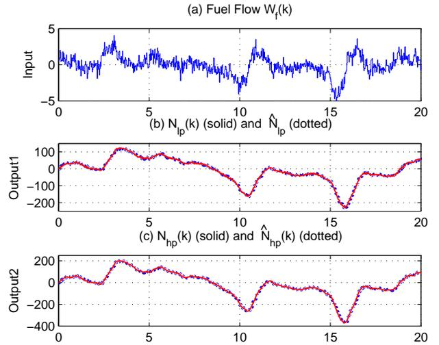
Fig. 3. Experiment: the input  $W_f$ , the outputs of the shaft speeds  $([N_{lp}, N_{hp}]^T)$  and their estimations  $[\hat{N}_{lp}, \hat{N}_{hp}]^T$  predicted by the observer  $K_0$ . Since the model is identified at a steady operating point, the data used here has been subtracted from the operating point equilibrium.
