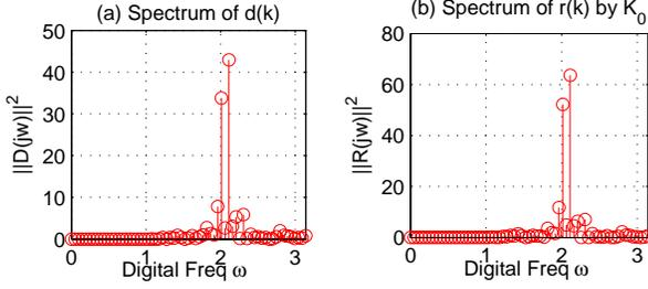
Fig. 4. (a) Disturbance spectrum and (b) its frequency estimation through 128-point FFT-based residuals spectrum analysis
